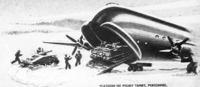
PLATOON OF PIGMY TANKS, PERSONNEL, SPARE FUEL AND AMMUNITION, CAN BE CARRIED IN NEW C-124 TRANSPORT
